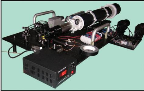
*Small Business Innovation Research funded by AFRL and completed by Nanohmics, Inc., generated an Optical Target Identification System (OTIS) for directed energy weapons research. Pictured is the OTIS setup used for field-based laser experimentation. (Photo courtesy of Ron Sullivan, Nanohmics)*
