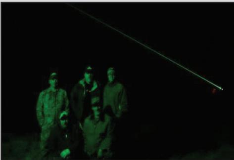
*The 532 nm scattered light from a diffuse target illuminates Nanohmics, Inc., researchers during the team's field-based laser experimentation. (Photo courtesy of Ron Sullivan, Nanohmics)*
