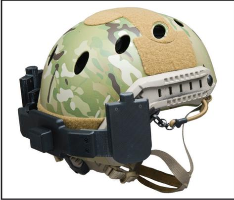
*AFRL Small Business Innovation Research contractor Appareo Systems developed this Head Attitude Tracking System (HATS) to provide warfighters with reliable heading reference in any outdoor environment. Pictured is a backside view of the HATS helmet with attached headset. (Air Force photo)*
