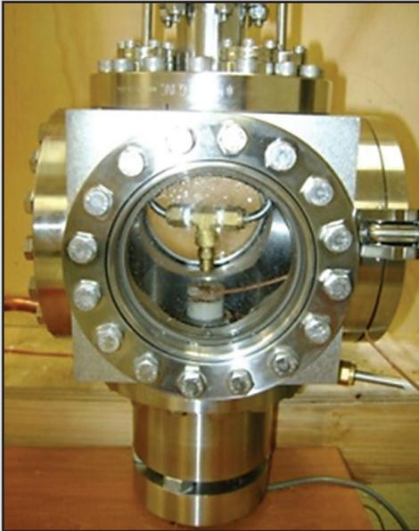
*North Carolina A&T State University—developed spray chamber for testing technologies that could enhance high-heat-flux heat transfer. (AFRL image)*
