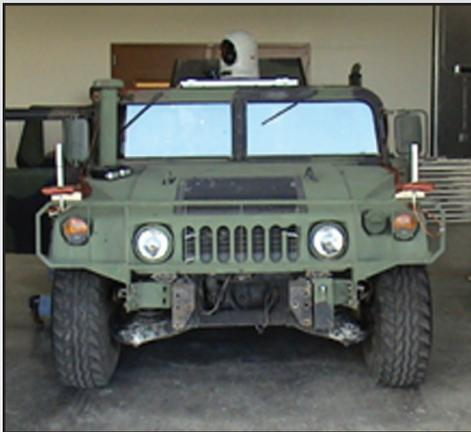
*High-mobility multipurpose wheeled vehicle equipped with FALCON, the Fast Airborne Laser Communications Optical Node, for demonstration testing in Albuquerque, New Mexico (AFRL image)*
