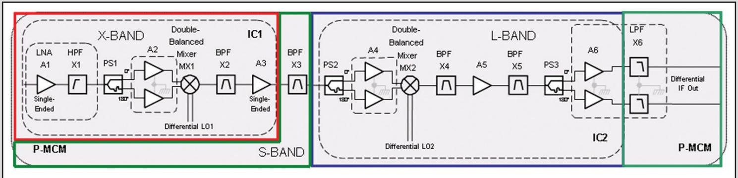
As part of supporting a Defense Advanced Research Projects Agency effort to create self-healing integrated circuitry, AFRL sensors scientists oversaw development of a wideband, 6-18 GHz receiver-on-a-chip with baseband outputs, the architecture of which is illustrated. (Air Force image)
