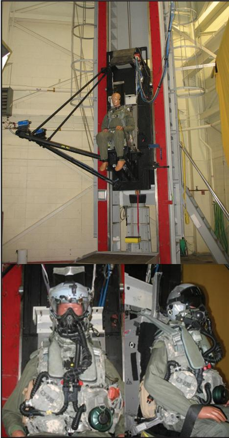
*A manikin fitted with a Joint Service Aircrew Mask and Joint Helmet-Mounted Cueing System facilitates AFRL's recent biodynamic evaluation of the protective equipment in terms of pilot neck loads. (Air Force image)*
