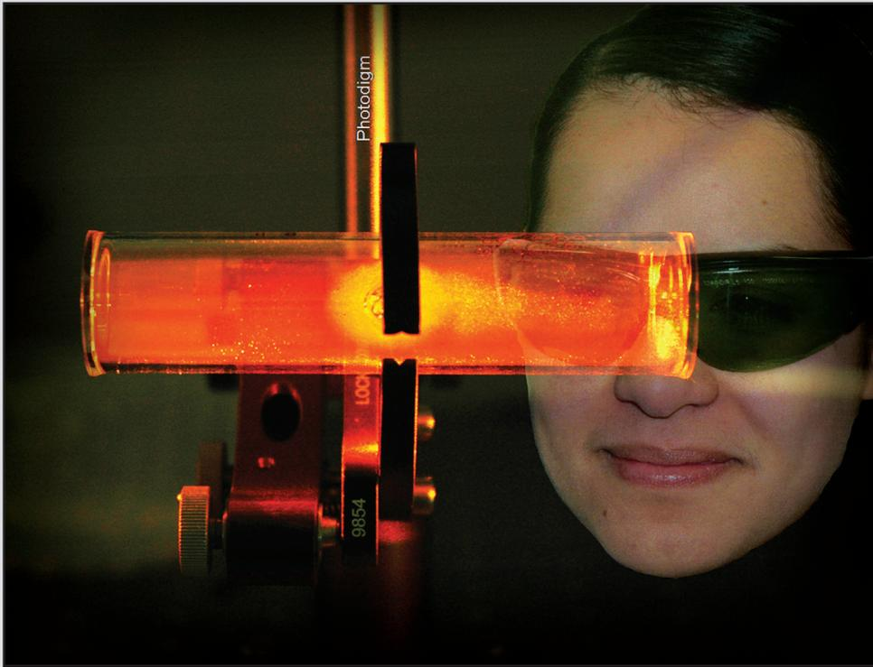
*Photodigm, Inc., engineer Judy Perez observes the faint, deep red glow of rubidium (Rb) vapor fluorescing under illumination of the company's new semiconductor laser, precisely tuned to match an electronic transition of Rb atoms. (Credit: Martin Achtenhagen)*
