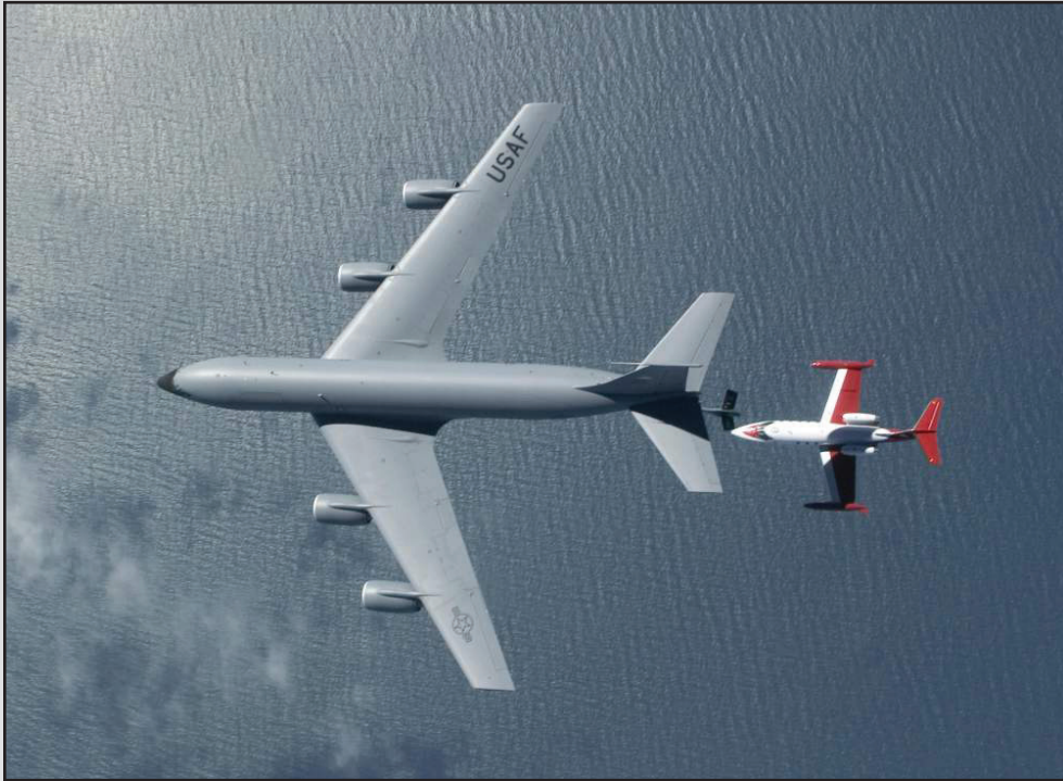
Pictured are the KC-135 Tanker and Calspan Learjet used during Automated Aerial Refueling flight tests. (Air Force image)
